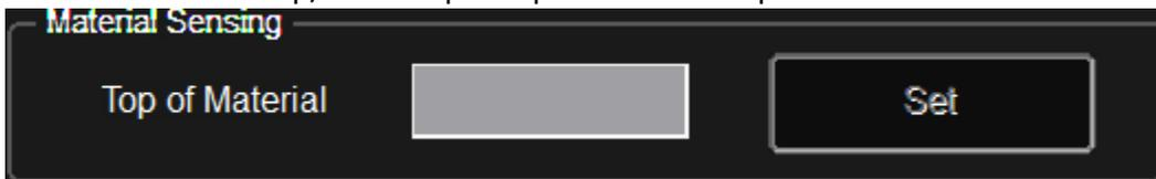
4. Then jog the Z-axis up and if the torch is not already at the start location, jog the torch to the start location and press the Set Plate Origin/Set Program Zero button.
