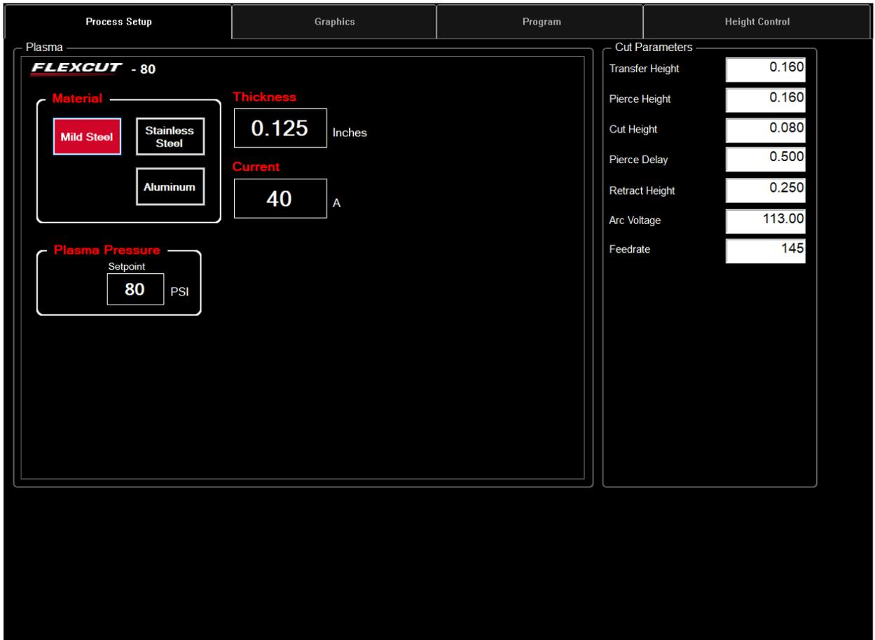
The screenshot displays the 'Process Setup' tab for the 'FLEXCUT - 80' plasma cutting system. The interface is organized into several sections:
