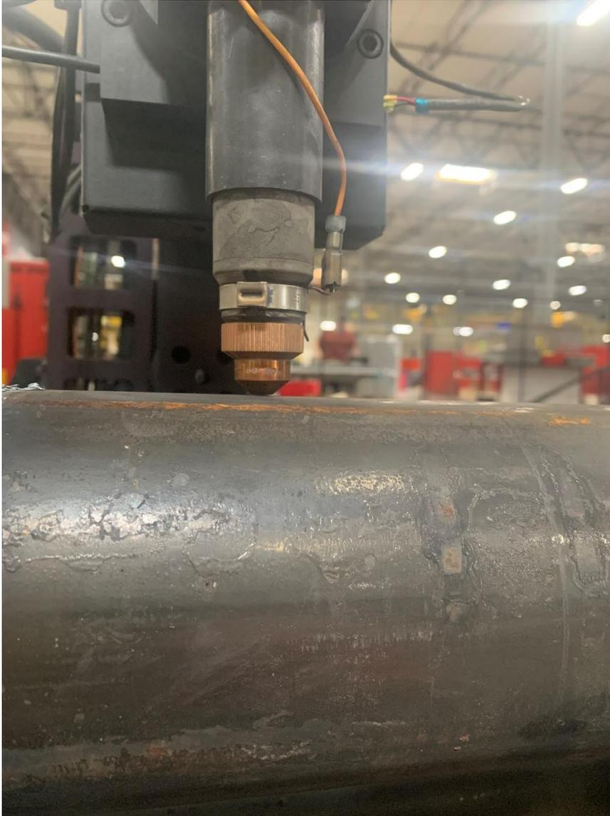
3. Go to the Plate Setup/Job Setup and press the **Set** top of material button.
